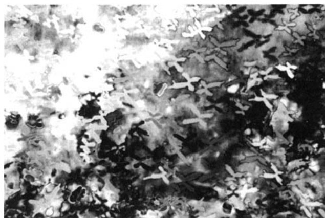
Figure 2. Butterfly dendrites of smectic B phase in coexistence with a nematic phase: 10 mol% CB5 in N at 24°C.
